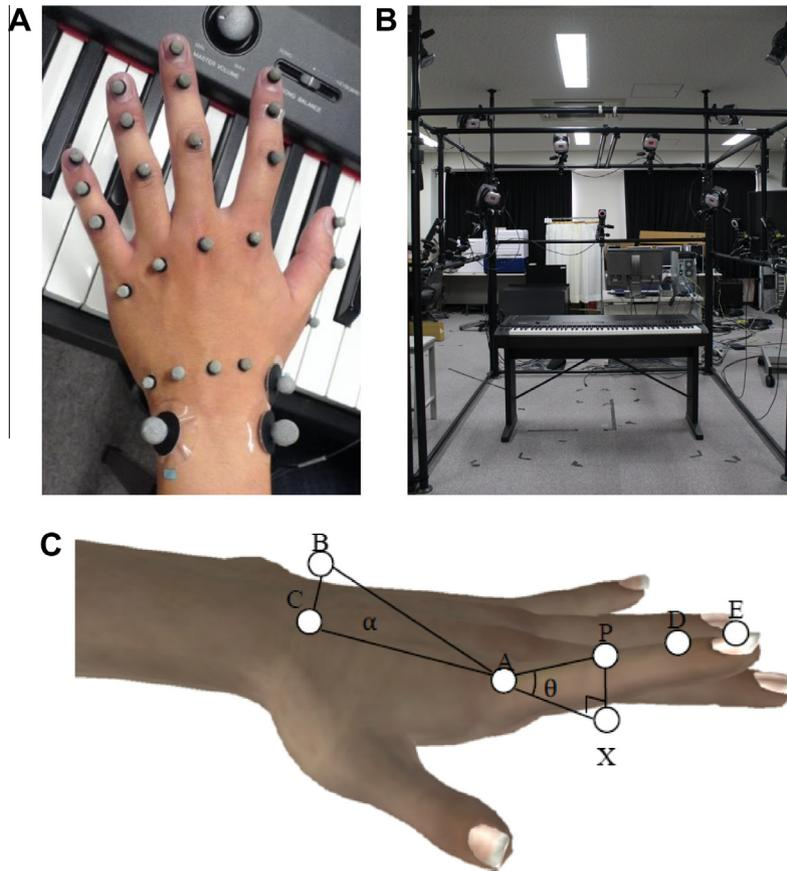
**Fig. 2.** (A) Reflective markers on the left hand. (B) The motion capture system consisted of 13 high-speed cameras. (C) The markers used to calculate the joint angle.
